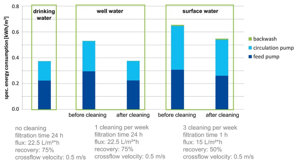
Figure 5. Energy consumption for different operation conditions
