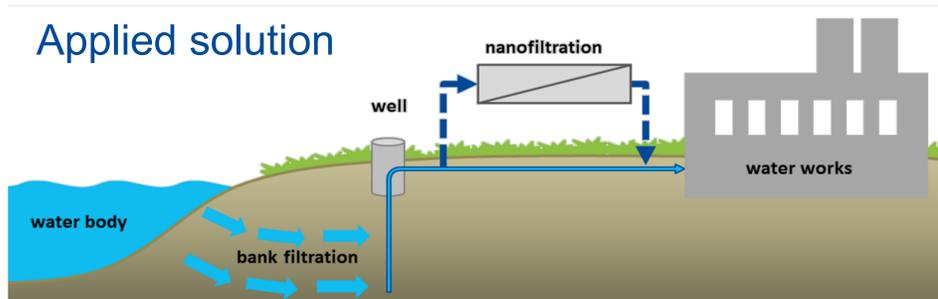
Figure 1. Bank filtration as natural pre-treatment for decentralized capillary NF with new developed LbL coated membrane
