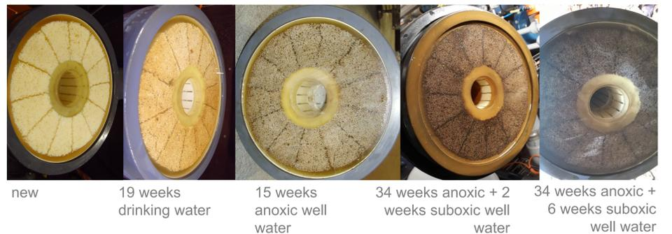
Figure 4. Irreversible impurities on membrane, after chemical cleaning
