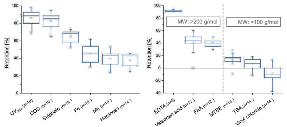
Figure 3. Retention of compounds (well water, flux  $22.5 \text{ L/m}^2 \text{ h}$ , rec 75%, cfv  $0.5 \text{ m/s}$ )
